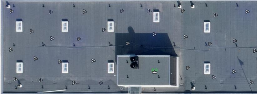
*In this example, the roof area is approximately 600 square metres and it is monitored by 30 sensors.*
